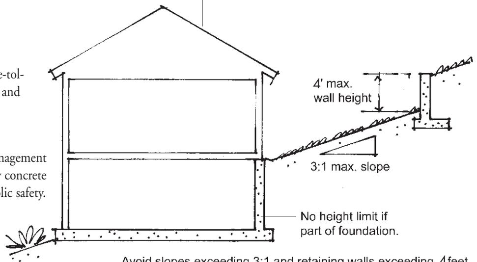
Avoid slopes exceeding 3:1 and retaining walls exceeding 4 feet.
