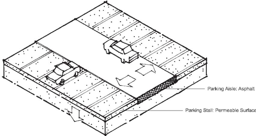
Parking stalls receive less wear and make good locations to increase infiltration through the use of permeable materials.
